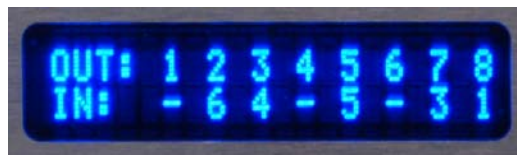
Figure 4: Routing status display (example)
